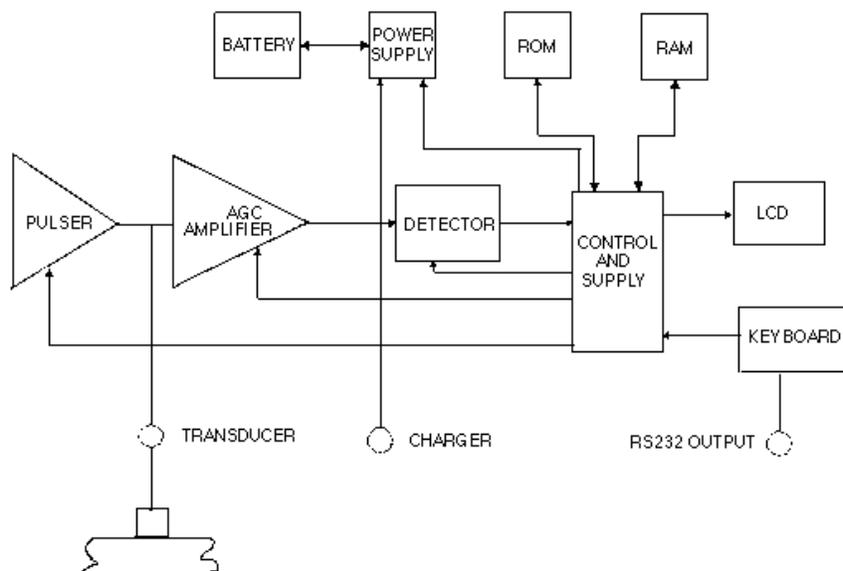
Figure A3: Ultrasonic Gauge Block Diagram
