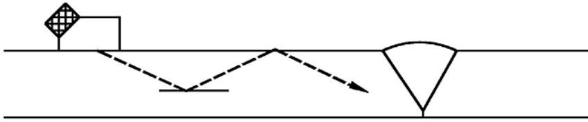
Figure A6: Angle Beam Lamination Inspection
