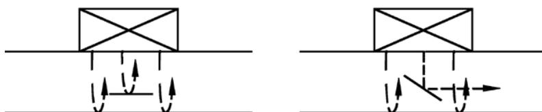
Figure A5: Straight Beam Lamination Inspection
