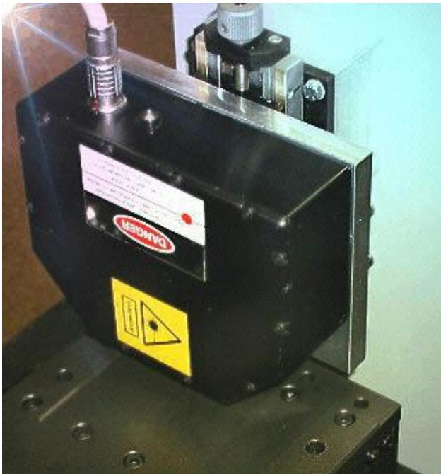
Figure A2: Laser Gauge System
