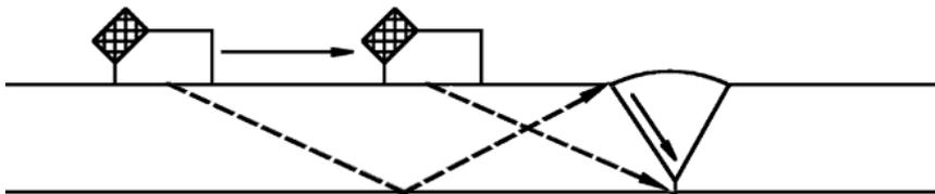
To determine the proper scanning area for the weld, the inspector must first calculate the location of the sound beam in the test material. Using the refracted angle, beam index point and material thickness, the V-path and skip distance of the sound beam is found. These values are illustrated in Figure A8. Once they have been calculated, the inspector can identify the transducer locations on the surface of the material corresponding to the crown, sidewall, and root of the weld.
