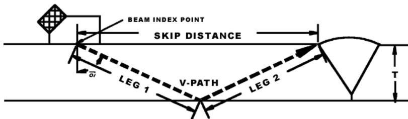
Figure A9: Reflector Components
