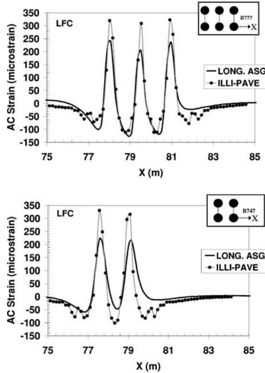
FIG. 9—Comparison of early-life longitudinal AC strains in LFC section.
