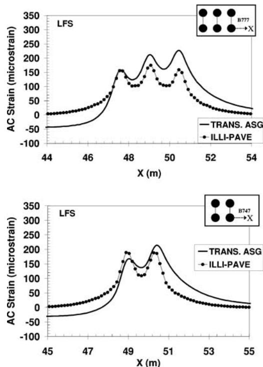
FIG. 12—Comparison of early-life transverse AC strains in LFS section.
