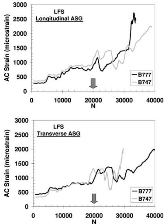
FIG. 8—Peak AC strains in LFS section during trafficking.
