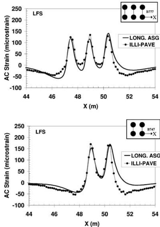
FIG. 10—Comparison of early-life longitudinal AC strains in LFS section.
