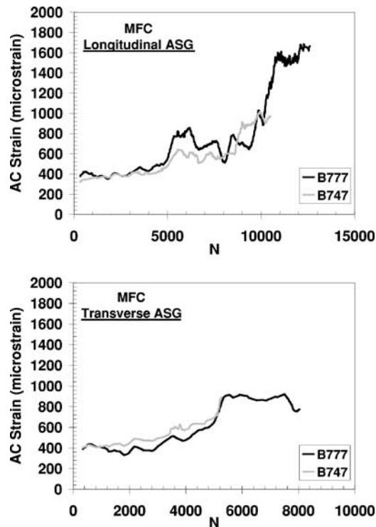
FIG. 5—Peak AC strains in MFC section during trafficking.
