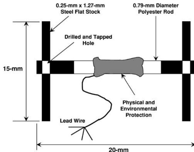
FIG. 2—Details of Asphalt concrete Strain Gage (ASG) used at NAPTF.
