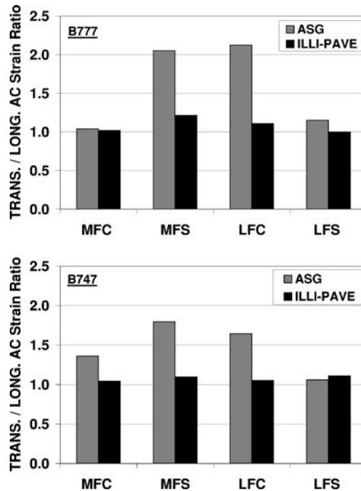
FIG. 13—Comparison of transverse-longitudinal AC strain ratios.
