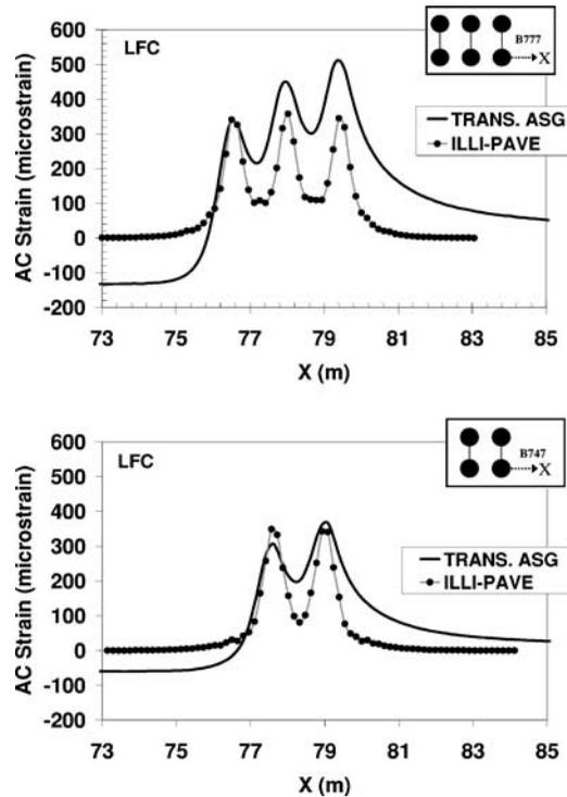
FIG. 11—Comparison of early-life transverse AC strains in LFC section.
