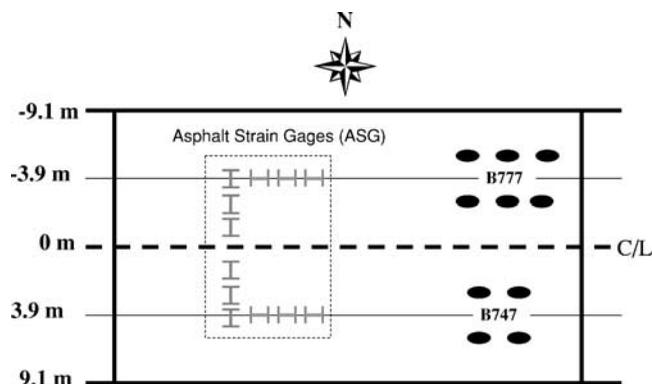
FIG. 3—AC strain gage installation at NAPTF.
